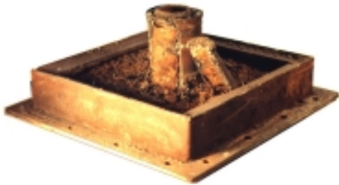
The interior of a sidewall circulating fan from a carburizing furnace showing extensive corrosion damage and fouling. A Spot•Cooler now keeps this fan running clean and cool.
