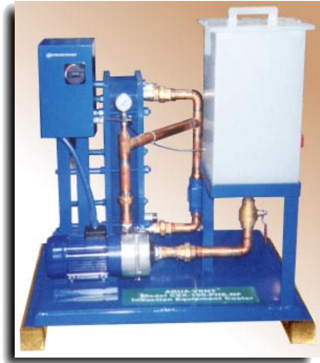
The Aqua-Vent® NFP-80 Non-Ferrous Cooling System with Thermostatic Mixing Valve and Tank Level Switch. Designed to provide 35 gpm at 80 psi and a cooling capacity of 80 kW.
